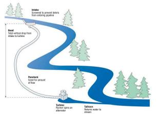
The key elements of a hydro power system are:
